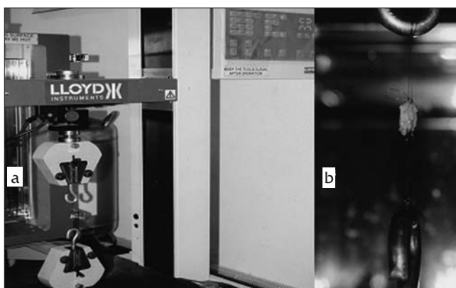
Figure 3. a. The tensile strength test machine (Lloyd Inst, UK), b: A progressively increasing force (in Newton units=N) was applied to the two ends of the section's including the LPS muscle and the tarsus which were tied to the hooks with 6.0 polyglactine
